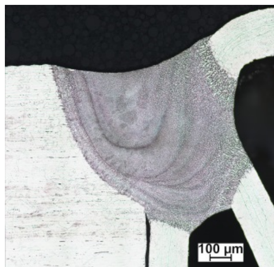
Fig. 9 The macrostructure of the EB welded joint
