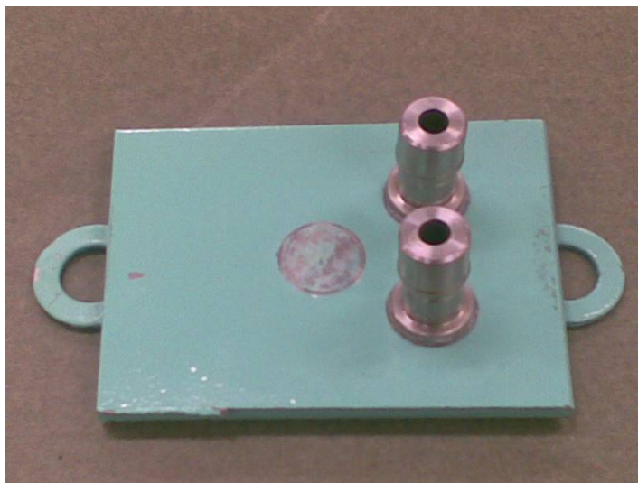
Fig. 15 Coating after Pull- Off test by dolly 20 mm diameter
