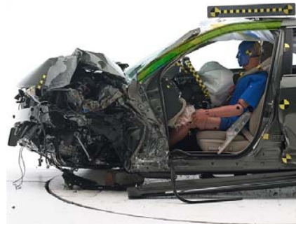
Fig. 16 Overlay of 2015 Camry A-Pillar Simulation on Actual Crash Photo
