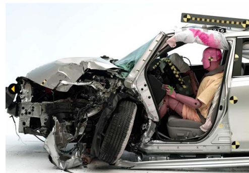
Fig. 6 2012 Camry Small Overlap Frontal Crash Results
