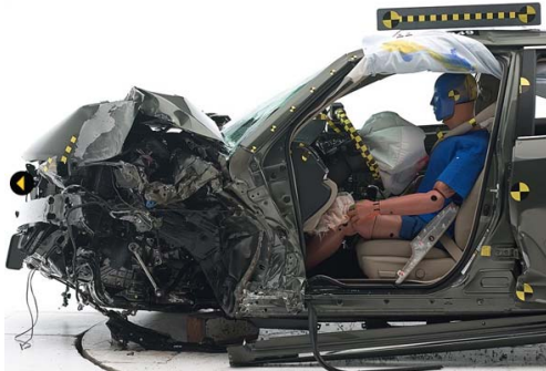
Fig. 7 2015 Camry Small Overlap Frontal Crash Results
