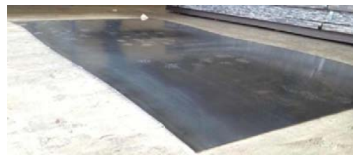
Fig. 3 Sample of edge waviness defect
