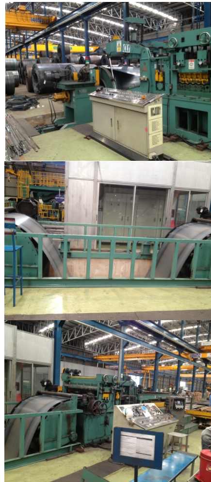
Fig. 2 Process of uncoil and shear of coil steel
