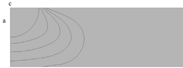
Fig. 13 The crack shape development for a deep semi-circular surface crack ( a/w=0.5 , a/c=1 ) under ductile tearing in biaxial load.
