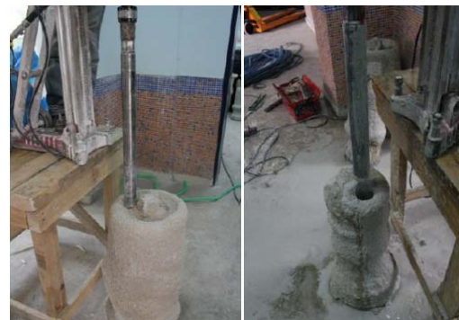
Fig. 5 Taking cores from the columns
