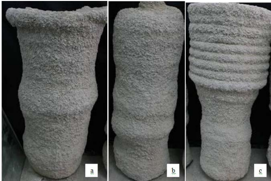
Fig. 4 JG columns produced in (a) 1 st Combination (b) 2 nd Combination (c) 3 rd Combination
