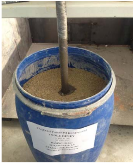
Fig. 3 Placing the sand into the experiment tank and the lowering process of the rod
