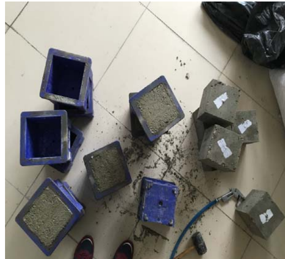
Fig. 6 Cube specimens after abstracting
