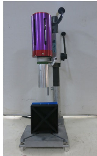
Fig. 8 Ultrasonic tube flanging specialized station
