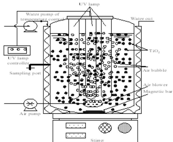
Fig. 1 Schematic of the photocatalytic batch reactor
