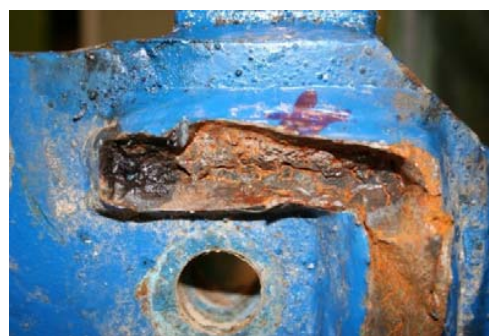
Fig. 1 Joint n. 2. Fracture surfaces covered with rust
