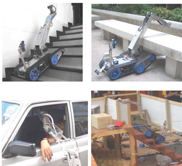
Fig. 11 CEO Mission II rescue robot testing under various conditions
