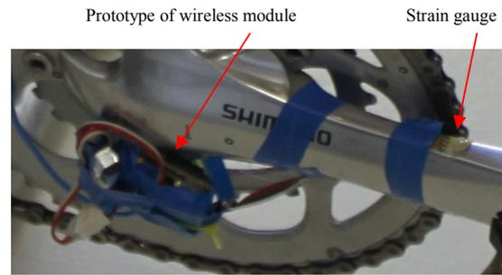
Fig. 5 Wireless strain gauge measurement of cranksforces
