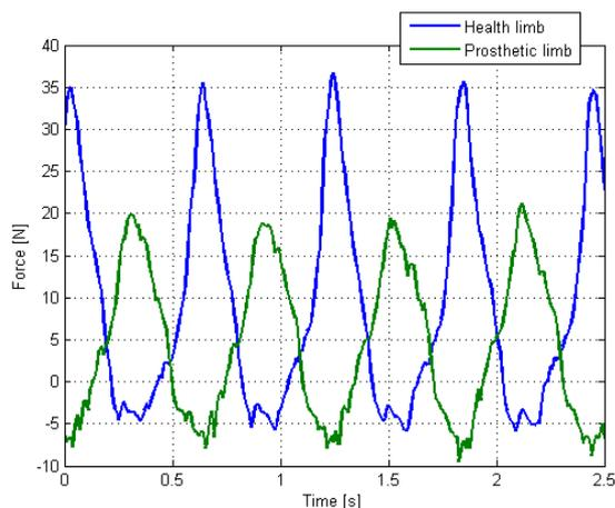
Fig. 12 Forces in the cranks – seated position, 167.5mm
