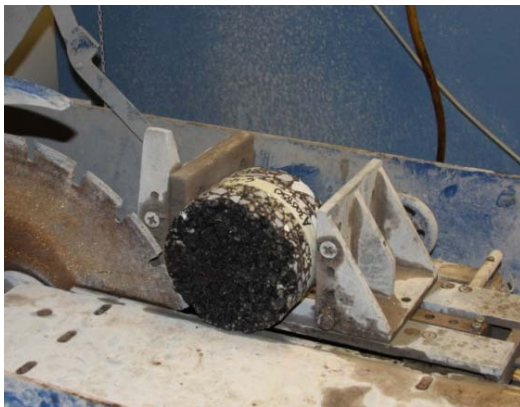
Fig. 2 Cutting a sample using a laboratory saw
