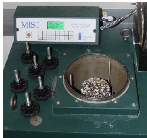
Fig. 4 MIST moisture conditioning device
