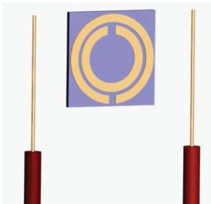
Fig. 2 Schematic diagram of the SRR placed between transmitting and receiving probes
