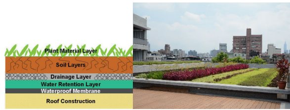
Fig. 2 The green roof configuration and environment images
