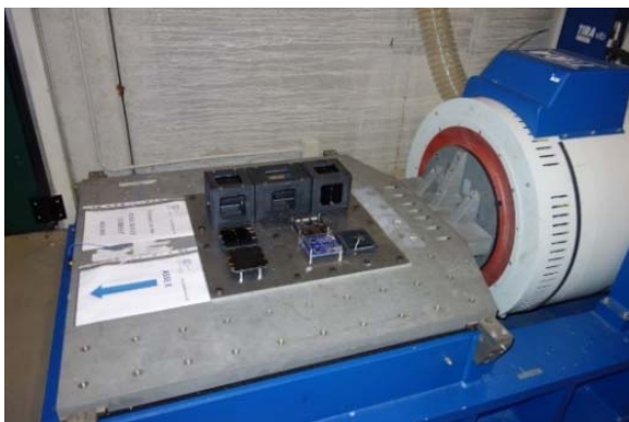
Fig. 8 CubeSat and modules installed on TIRA Shaker
