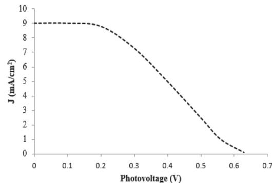
Fig. 3 Current density-voltage Characteristics for organic dye
