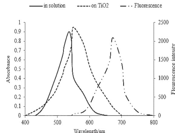
Fig. 2 UV-Vis absorption and fluorescence spectra of dye
