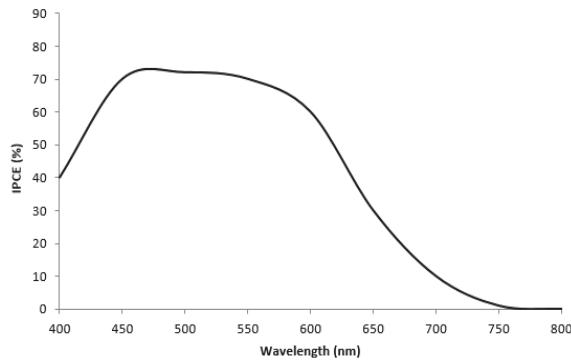
Fig. 4 Photo-to-current action spectra of synthesized dye
