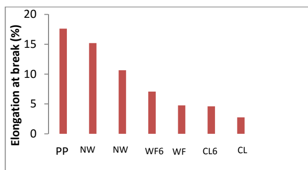
Fig. 6 Elongation at break for different date wood flour composites
