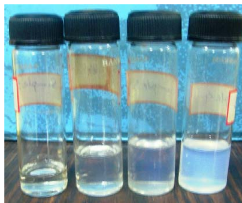
Fig. 4 Photographs of prepared nanoemulsions with Tergitol 15-S-5, Tergitol 15-S-7, Tergitol 15-S-9 and Tergitol 15-S-12 (From left to right)
