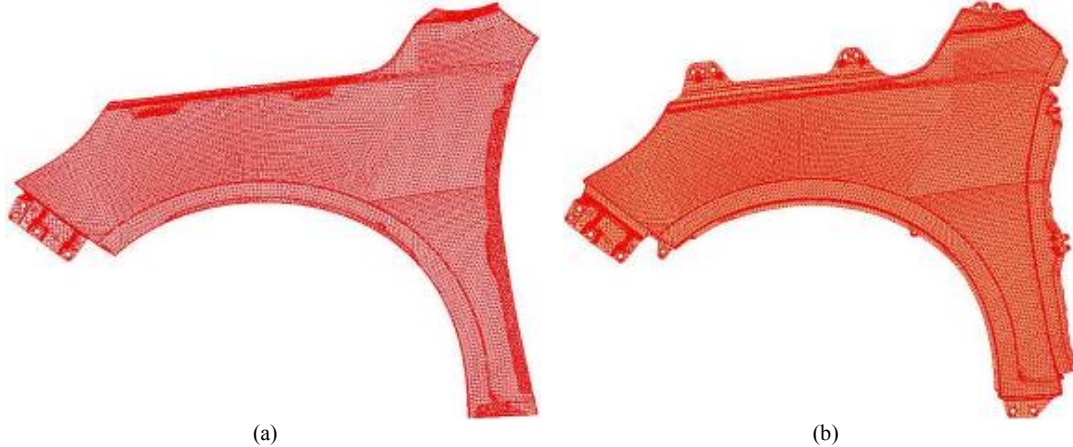
Fig.4 Flattening of fender (a) three dimensional surface, (b) flattening result
