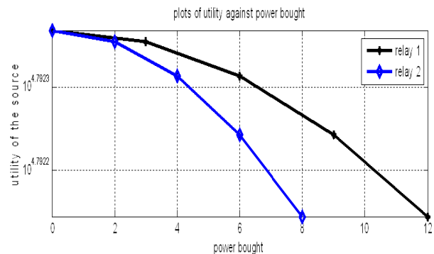
Fig. 8 Plots of variation of the utility of the source node with the power bought from the relay node
