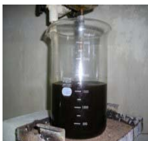
Fig. 4 HNO 3 Digestion of Rare Earth Hydroxide
