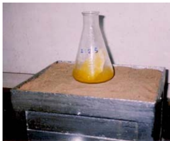
Figure (2) Hydrochloric Acid Dissolution
