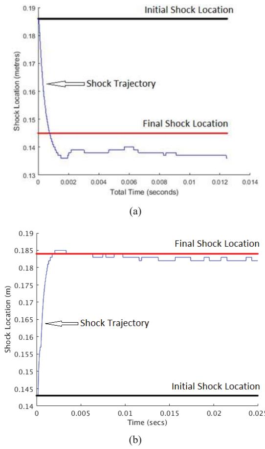
Fig. 5 (a) Shock Location versus Time for an external compression wave perturbation (b) Shock Location versus Time for an external expansion wave perturbation
