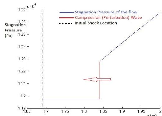
Fig. 1 Flow schematic for a compression (perturbation) wave travelling upstream
