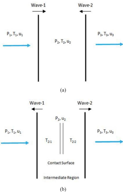
Fig. 2 (a) Flow schematic just before the instant of wave interaction
