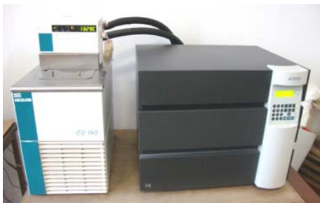
Fig. 3 Apparatus Holometrix 2300 for determination of thermal conductivity
