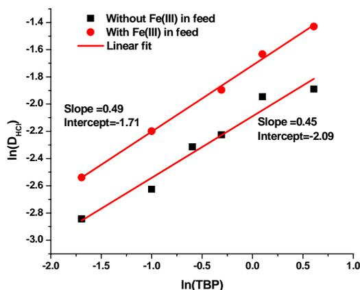
Fig. 6 log-log relation between distribution coefficient of HCl extraction with and without Fe(III) in feed (TBP concentration varied from 5-50%, 40% n-decanol in org phase, Initial Feed 8N HCl,  $C_{Fe(III)}(0)=1000\text{ppm}$ )
