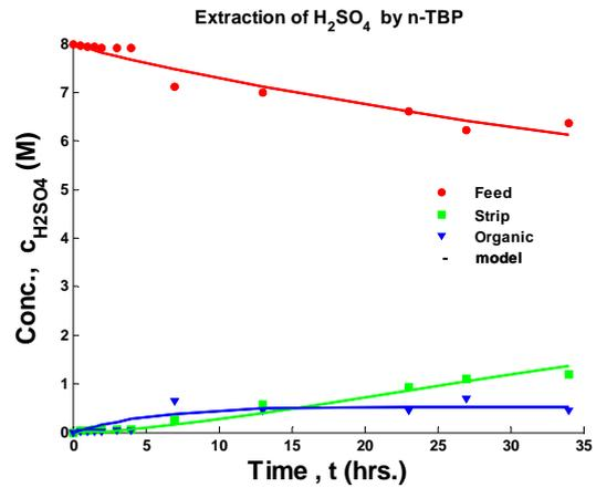
Fig. 4 Experimental concentration profile of  $H_2SO_4$  and theoretical results from the fitting the model (10% TBP, stirrer rpm =100, 40% n-decanol, Initial feed 8(M)  $H_2SO_4$ ,  $C_{Fe(III)}(0)=1000\text{ppm}$ )
