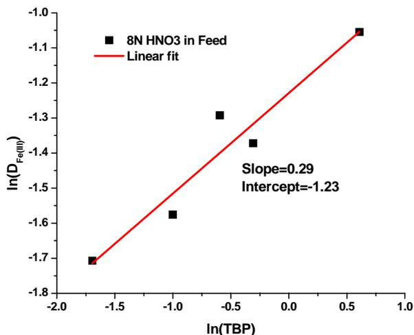
Fig. 9 log-log relation between distribution coefficient of  $HNO_3$  extraction (TBP concentration varied from 5-50%, 40% n-decanol in org phase in paraffin, Initial Feed 8N HCl,  $C_{Fe(III)}(0)=1000$ ppm)
