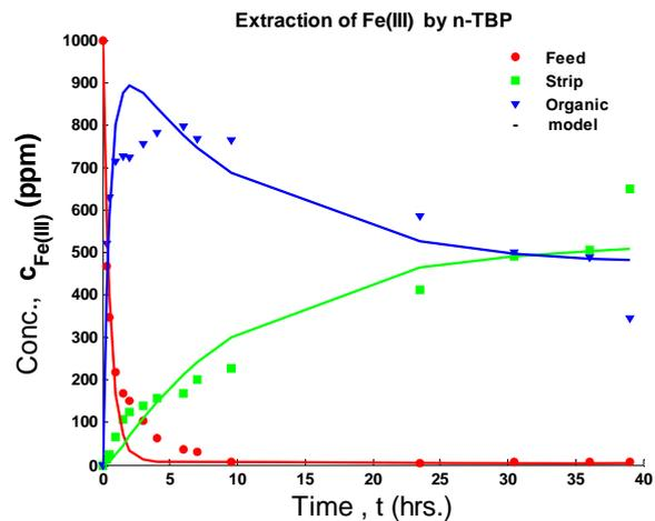
Fig. 5 Experimental concentration profile of Fe(III) and theoretical results from the fitting the model (10% TBP, stirrer rpm =100, 40% n-decanol in org phase, Initial Feed 8N HCl,  $C_{Fe(III)}(0)=1000\text{ppm}$ )
