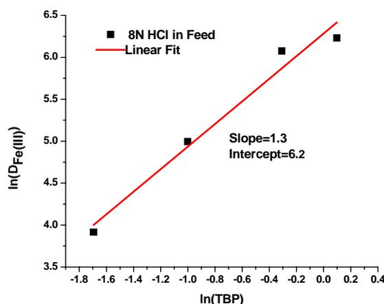
Fig. 7 log-log relation between distribution coefficient of Fe(III) extraction (TBP concentration varied from 5-50%, 40% n-decanol in org phase in paraffin, Initial Feed 8N HCl,  $C_{Fe(III)}(0)=1000\text{ppm}$ )
