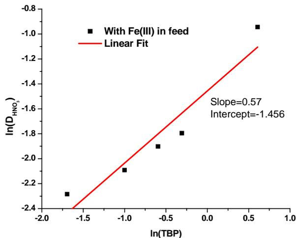
Fig. 8 log-log relation between distribution coefficient of  $HNO_3$  extraction (TBP concentration varied from 5-50%, 40% n-decanol in org phase in paraffin, Initial Feed 8N HCl,  $C_{Fe(III)}(0)=1000$ ppm)
