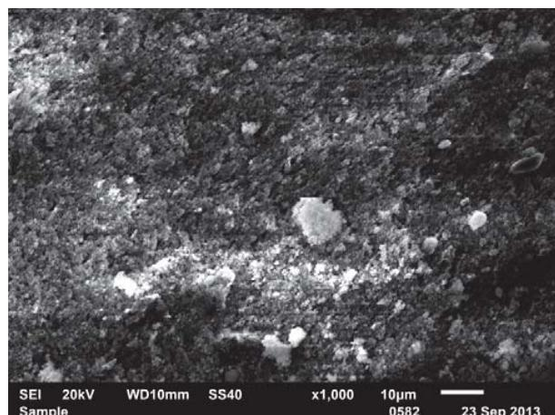
Fig. 2 Electron micrograph of thermal treated catalyst
