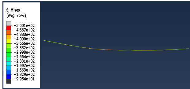
Fig. 7 Stress distribution for cable wire (case2)
