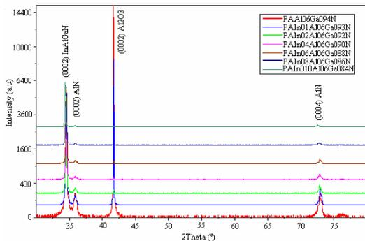
Fig. 1 XRD Phase analysis of  $\text{In}_x\text{Al}_y\text{Ga}_{1-x-y}\text{N}$  quaternary alloys
