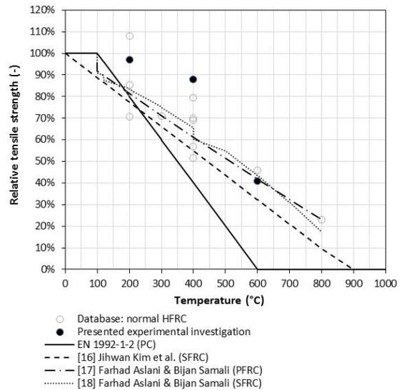
Fig. 6 Relative splitting tensile strength diagram
