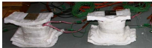
Fig. 2 HFRC specimens during the heat treatment
