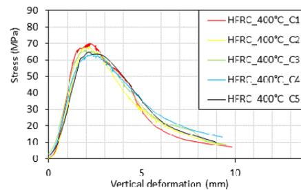
(c) Stress-displacement diagram of HFRC at 400°C
