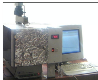
Fig. 2 Fabricated heating chamber around TPA cross head
