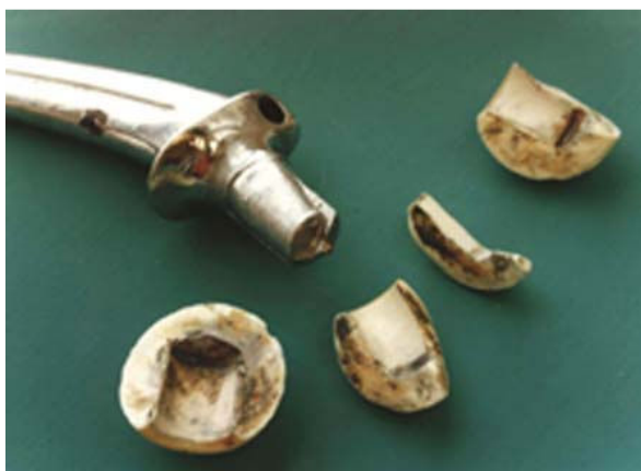
Fig. 1 In vivo destructed ceramic heads of total hip joint endoprosthesis
