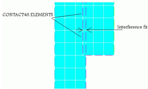
Fig. 1. element and mesh combination
