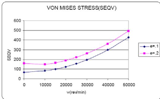
Fig. 6 Variation of maximum von misses stress versus speed of rotation for overlap=10 cm
