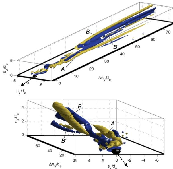
Fig. 4 Streamwise reconstruction of vorticity for isosurfaces of  $\Omega = \pm 1.3$  for  $\alpha = 30^\circ$ ,  $d_e = 5.8 \text{ mm}$ ,  $\phi = 90^\circ$ . The key structures A, B and B' are also highlighted
