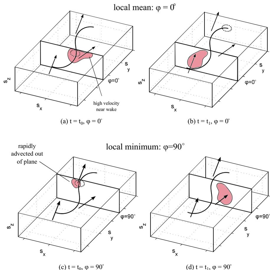
Fig. 7 The structures observed in the PIV measurement planes at the two phase angles at two times  $t_0$  and  $t_1$ . The bubble location and path are provided, and the arrows indicate the motion of the shed fluid in the bubble wake
