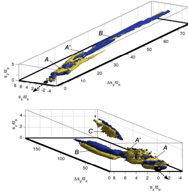
Fig. 6 Streamwise reconstruction of vorticity for isosurfaces of  $\Omega = \pm 1.3$  for  $\alpha = 30^\circ$ ,  $d_e = 5.8\text{mm}$ ,  $\phi = 0^\circ$ . The key structures  $A$ ,  $A'$ ,  $B$  and  $C$  are also highlighted
