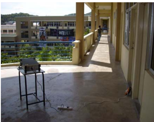
Fig. 13: A depiction virtually covering measurement surroundings for both models II and III. Notice the passageway for model II, which continues to the left looking straight up through the passage. This passage is approximately 64.008m long (measuring from the receiver location to the extreme of the passage, looking right up).
