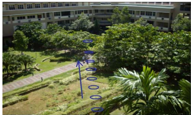
Fig. 15: Additional depiction of the ground and surrounding area to Fig. 14. The circles give an indication of the several transmit points, while the arrow points to the direction of increase in distance from the fixed receiver (i.e., the stationary receiver positioned up at level 4 of building from where this picture was taken).
