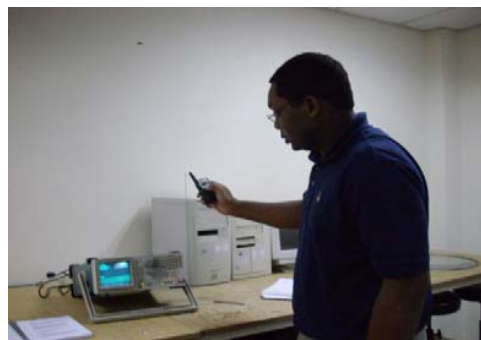
Fig. 9: Emmanuel Ojakominor carries out preliminary checks on transmit and receive devices before commencing actual measurements. Notice the transmit device (walkie-talkie, model T-388, with output power approximately 0.5W) and the receive equipment (Tektronix 2711 spectrum analyser along with a simple telescopic antenna)
