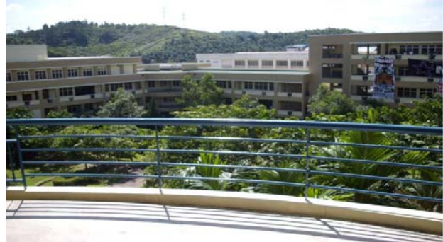
Fig. 14: A depiction of the ground and surrounding area corresponding to model III. Notice the foliage, which may well have shadowing effects on radio paths between a transmit spot on the ground area and the receiver located up at level four of building.
