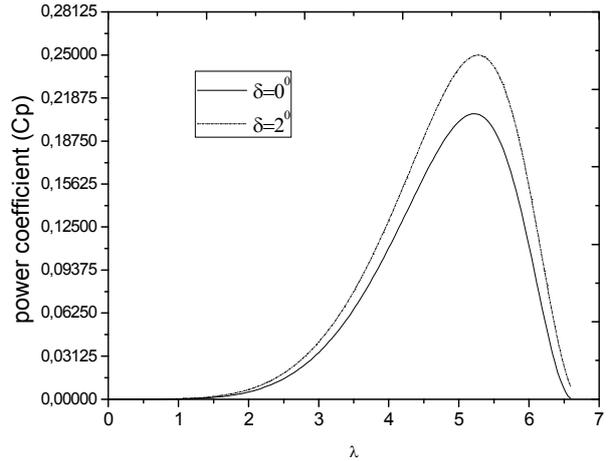
Fig. 10 Comparison of the power coefficient for fixed and pitched blade rotor
