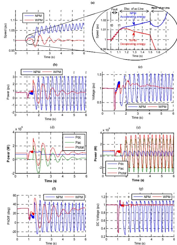
Fig. 12 (a) Generator speed (b) Generator active power output (c) Generator terminal voltage (d) AC ( $P_{ac}$ ), DC ( $P_{dc}$ ) and total ( $P_{total}$ ) power transfer WPM (e) AC ( $P_{ac}$ ), DC ( $P_{dc}$ ) and total ( $P_{total}$ ) power transfer NPM (f) Transmission angle ( $P_{HDiff}$ ) between two ends (g) DC Voltage
