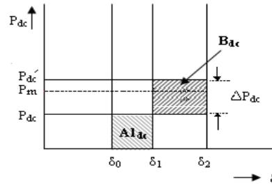
Fig. 10 Equal area criteria for DC control
