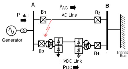
Fig. 3 Parallel AC-DC system
