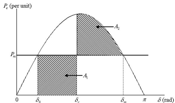
Fig. 7 Power-angle curve for equal area criterion.
