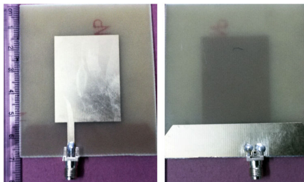
Fig. 9 Prototype of the proposed square monopole UWB antenna
