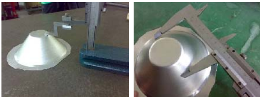
Fig. 6 Diameter measurements along the contour layers
