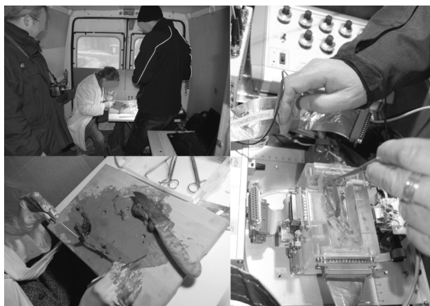
Fig. 3 (upper left) Experimental conditions, (lower left) insulation of the left vagus nerve segment, (right) installation of the left vagus nerve segment into the cuff
