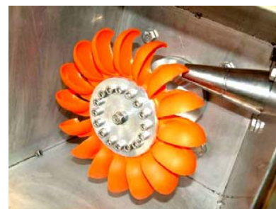
Fig. 1 Sketch of the flow in a Turgo turbine (up) and Turgo runner (down)
