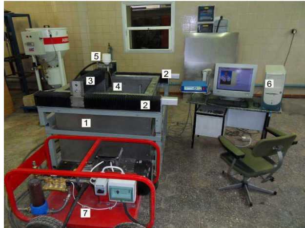
Fig. 2 General view of test stand for spatial material machining with high pressure AWJ: 1 – frame, 2 – y direction slideways, 3 – x direction slideway, 4 – abrasive-water jet working head, 5 – abrasive feed container, 6 – steering PC computer, 7 – high-pressure water pump type As500/15A
