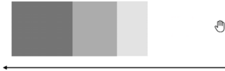
Fig. 1 Illustration of the system: The hand is on the right, and the three zones to reach on the left. The smallest zone is the one that is closest to the subject, the biggest is the farthest. The swipe gesture is oriented from the right to the left, as expressed by the axis on the bottom of the figure
