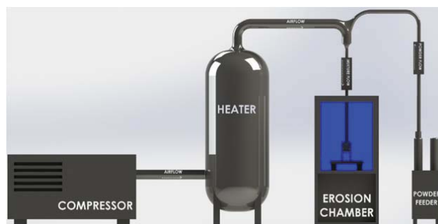
Fig. 2 Schematic representation of the high temperature erosion testing rig
