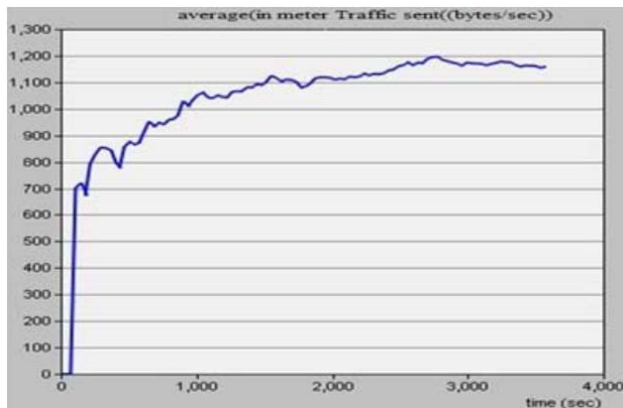
Fig. 4 Average WiMAX Throughput of Single Smart Meter
