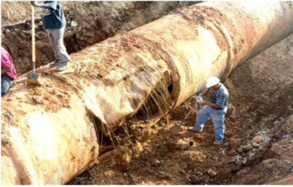
Fig. 2 Transient-caused failure, Super-aqueduct of Puerto Rico
