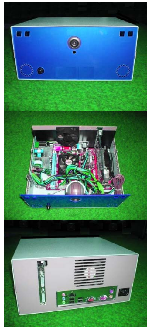
Fig.16: Set-top-box used by UNTreF.
