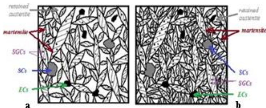
Fig. 7 A schematic of the microstructural development between the room temperature quenching (a) and the end of the SZT (b), with particular attention to the formation of SGCs
