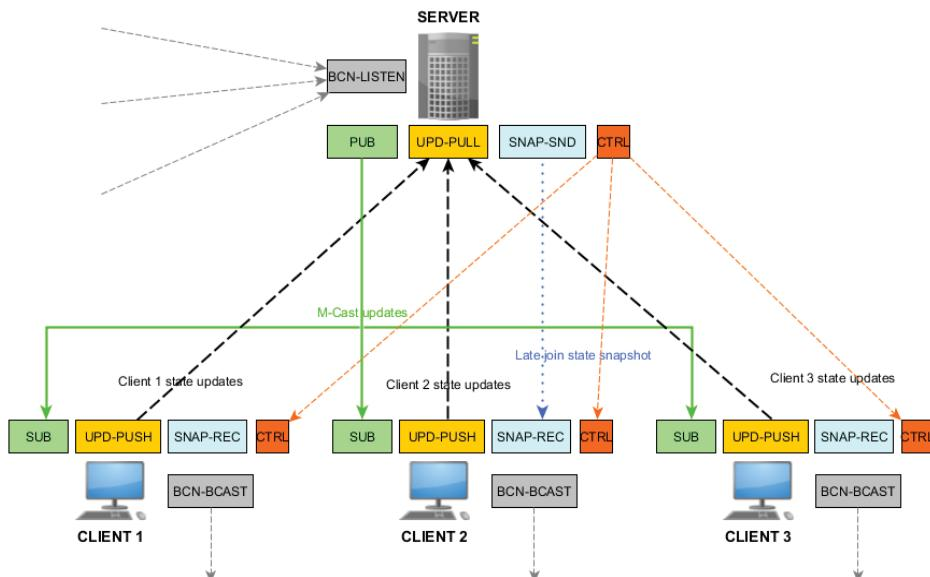
Fig. 4 Communication Channels of the Simulator Nodes
