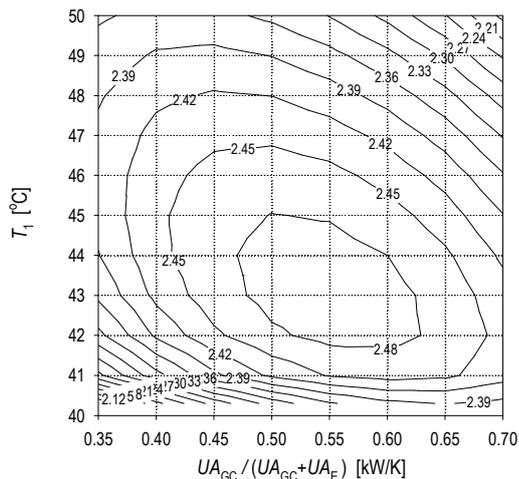
Fig. 3 Heating COP of carbon dioxide heat pump over the change of two independent variables when  $T_{HO}=90^\circ\text{C}$
