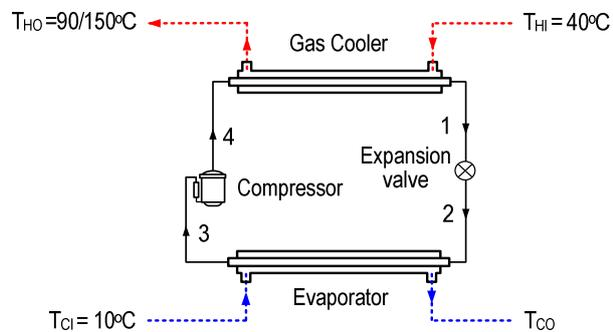
Fig. 1 Schematic diagram of a heat pump cycle
