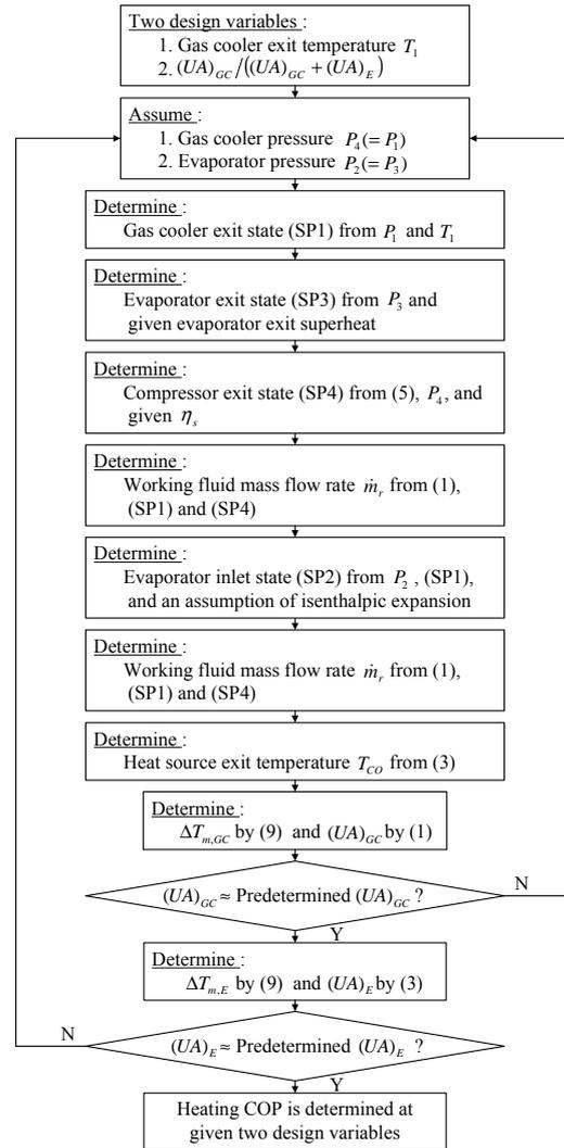
Fig. 2 Calculation procedure
